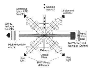
The SP2 measures both scattering and incandescence from individual particles containing rBC that are illuminated with a 1064 nm (near-IR) laser beam. The incandescence intensity is proportional to the amount of rBC mass. Calibration of the incandescence intensity is provided using size selected Fullerene soot.
