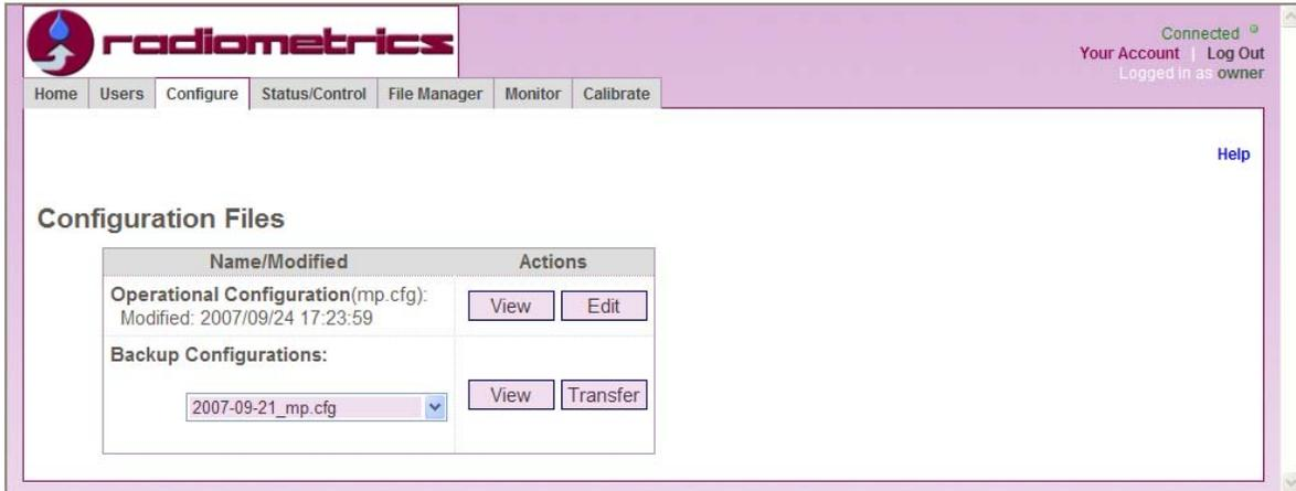
Figure 3. The radiometer *mp.cfg* file can be viewed, edited and transferred on this tab.
