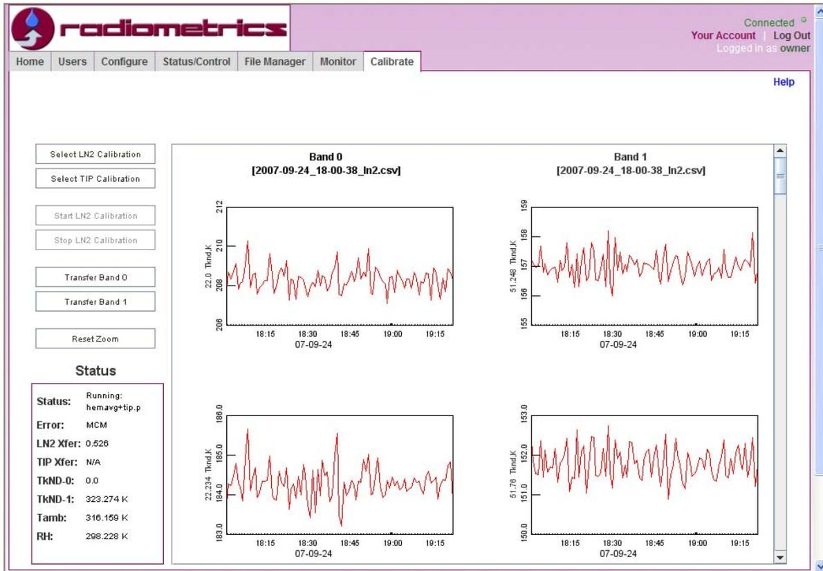
**Figure 9. The Calibrate tab allows liquid nitrogen (LN2) calibration control. It also allows TIP and LN2 calibration time series display and click and zoom data selection and transfer.**
