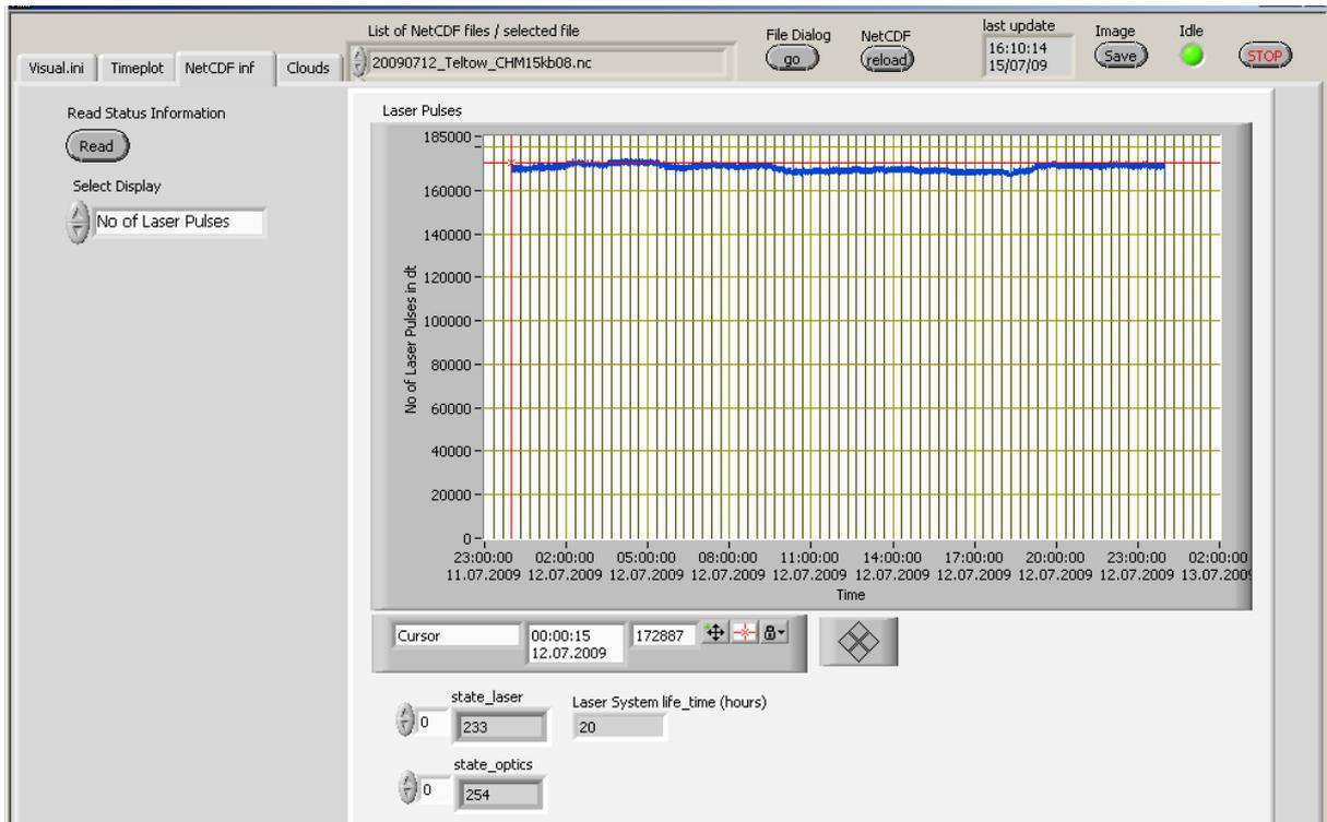
Figure 11: Laser control – If the No. of laser pulses are decreasing the laser diode is getting old.
