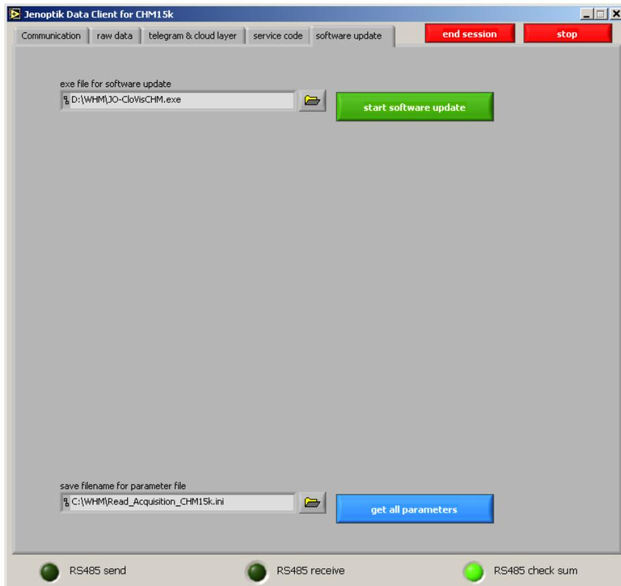
First, a file must be chosen in the field "exe file for software update". After pressing the (green) button "start software update" the update transmission to the CHM15k starts.
