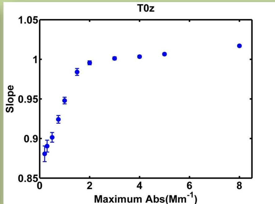
*Slopes of the correlation between light absorption coefficients at 880nm measured by AE33 with PM10 and PM2.5 inlets, as a function of the maximum absorption used in the regression.*
