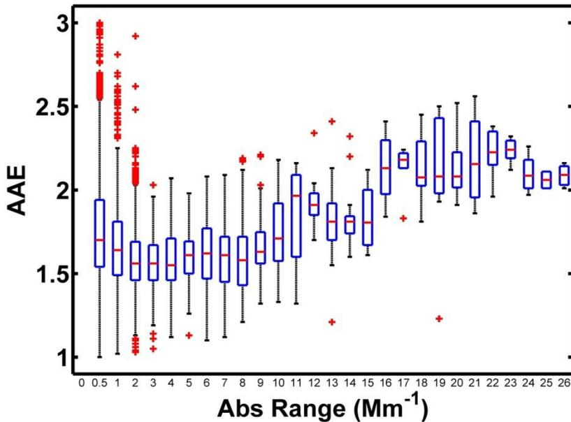
*Plots of AAE for different ranges of absorption coefficients for PM10 inlet.*
