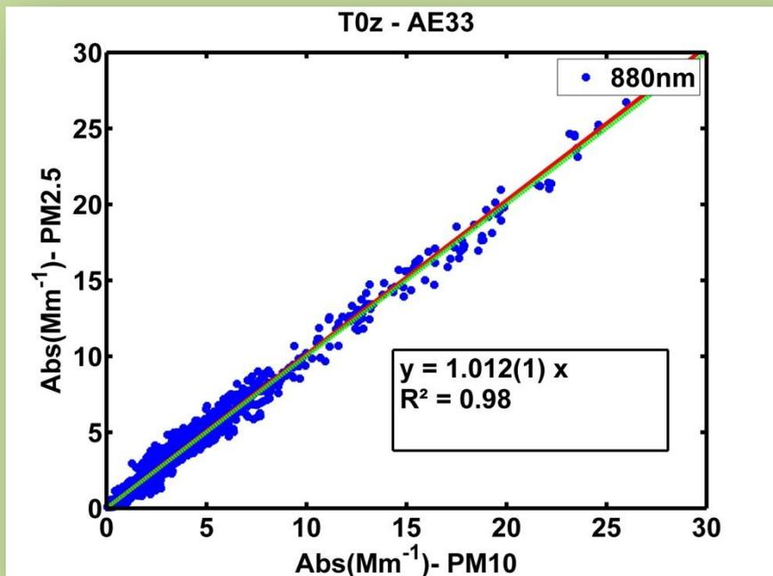
*Comparison of the light absorption coefficients at 880nm between AE33 with PM10 and PM2.5 inlets, showing 30 min averages of data compensated for the loading effect and multiple scattering.*
