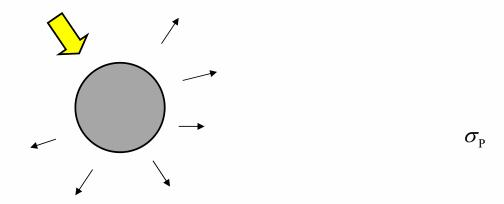
An illuminated spherical particle with a known Stokes diameter (latex particle) and a known refractive index gives a certain particle scattering
