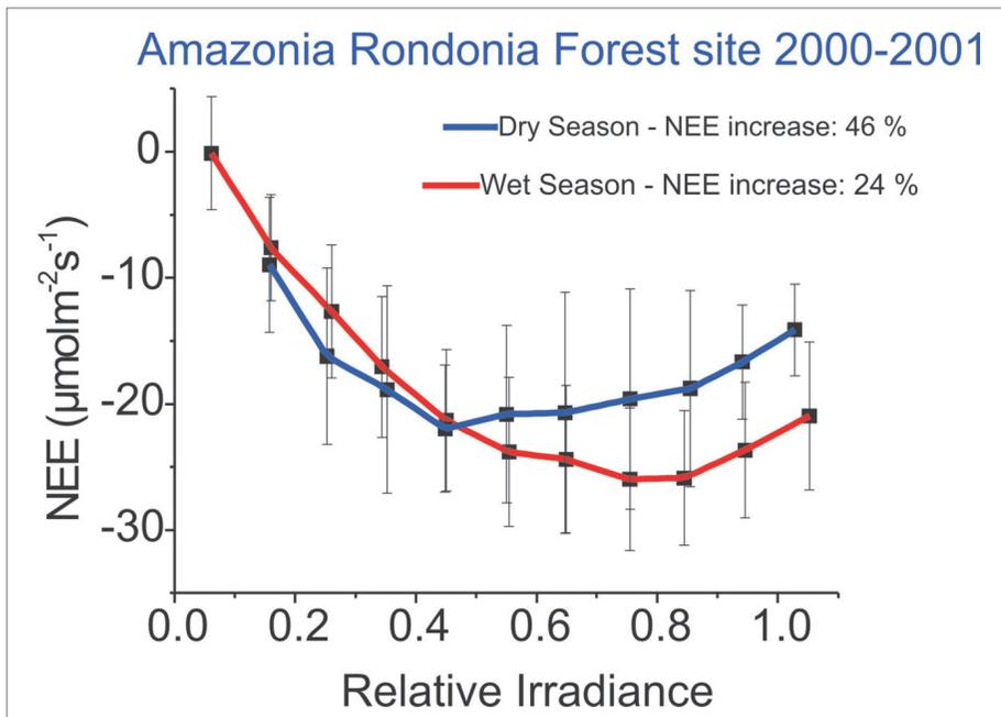
**Figure 2.** Net ecosystem exchange (carbon flux in  $\mu\text{mol m}^{-2}\text{s}^{-1}$ ) as a function of aerosol loading in the atmosphere expressed as the relative irradiance index. Note that negative values of NEE correspond to net ecosystem uptake, and that relative irradiance index decreases with increasing AOT. For details, please refer to Oliveira et al. [6].
