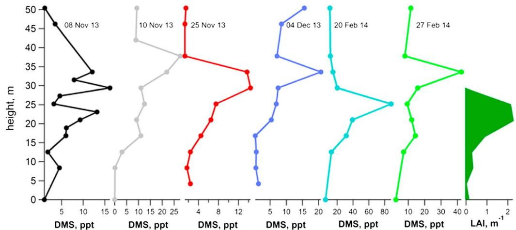
**Figure 6.** Example of high vertically resolved DMS mixing ratio measurements by GC-MS during the afternoon (13:00–15:00) on the K34 tower made between November 2013 and February 2014. Also shown are vertically resolved measurements of leaf area index (LAI). Note the buildup of DMS near the top and just above the 30 m canopy with mixing ratios up to 80 ppt.
