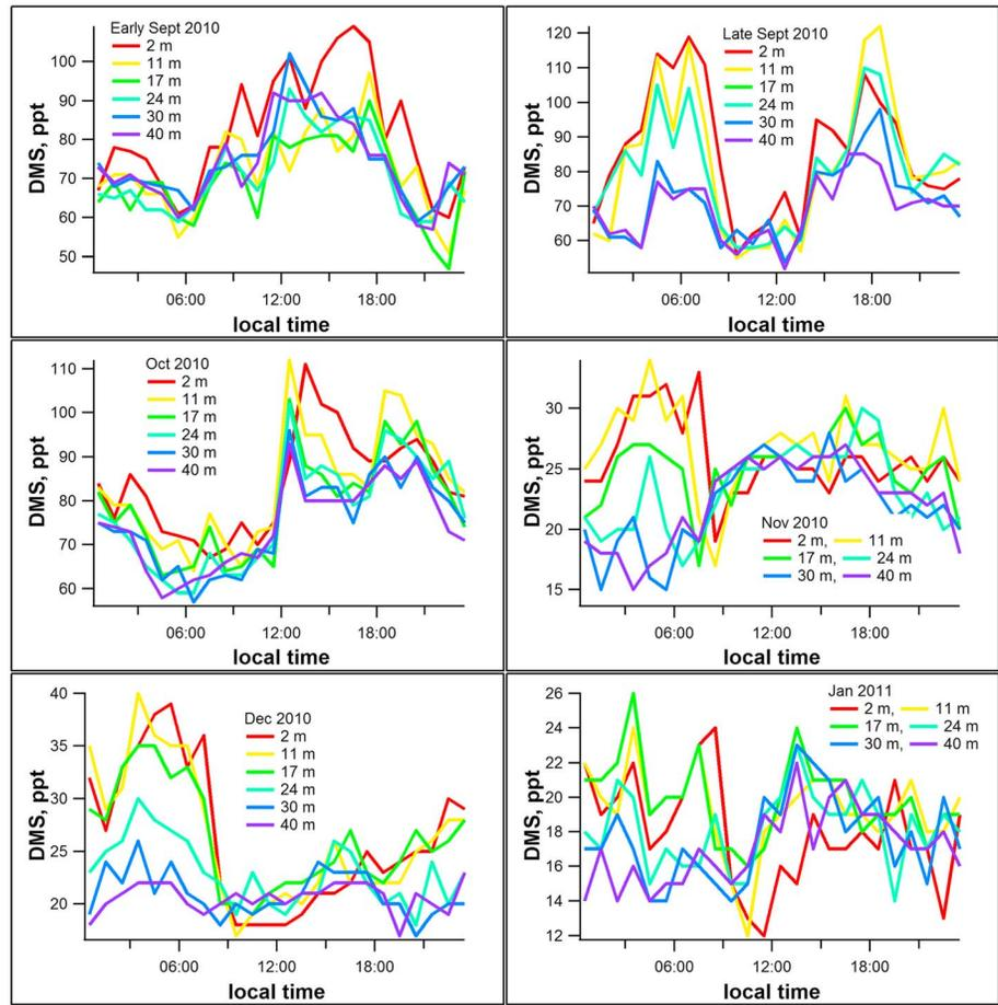
**Figure 3.** Mean diel patterns in ambient DMS mixing ratios at the TT34 site within and above the 30 m canopy between September 2010 and January 2011. Note the ambient mixing ratio enhancements within the canopy during the afternoon and evenings as well as the nocturnal buildup of ambient DMS mixing ratios within the canopy during some periods.
