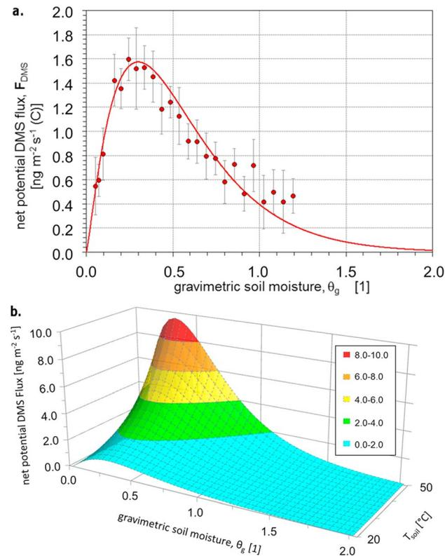
**Figure 2.** Net potential DMS flux from a soil sample collected from the Surinam Amazon as a function of (a) gravimetric soil moisture and (b) modeled gravimetric soil moisture and soil temperature by the use of a  $Q_{10}$  value of 2.06. Note that the error bars for gravimetric soil moisture are in the range of the size of the data points.
