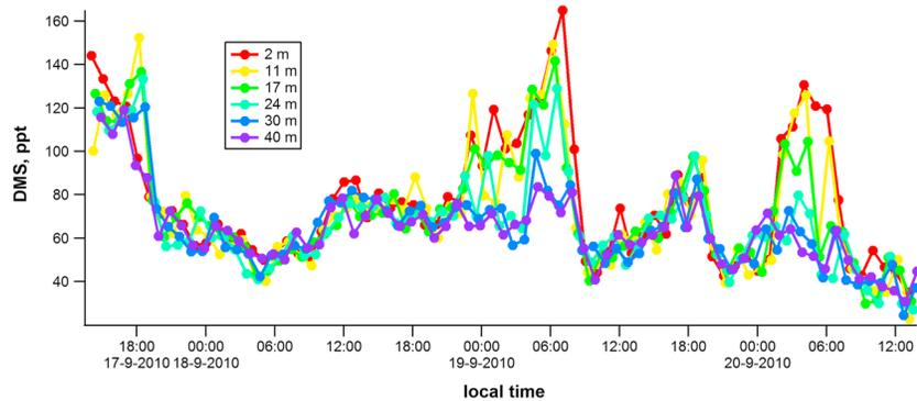
**Figure 4.** Example time series plots showing real-time ambient DMS mixing ratios within and above the canopy at the TT34 tower in central Amazon during the dry season (from 17 September to 20 September 2010). Note the buildup of DMS mixing ratios in the afternoon and during the night and early mornings just prior to sunrise within the canopy (height < 30 m).
