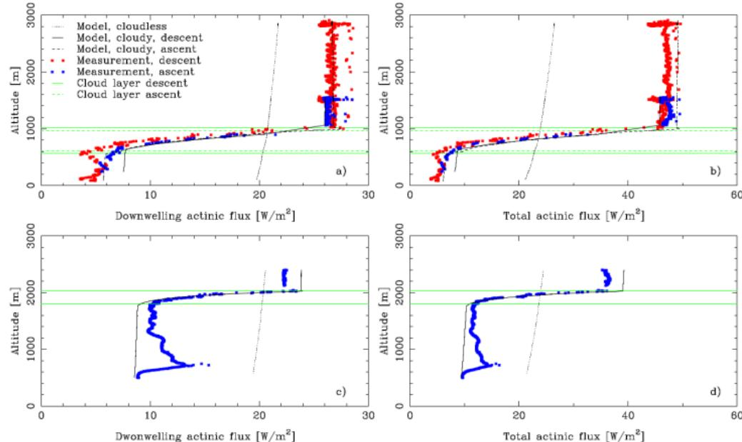
The actinic flux as measured by instruments on a Partenavia P68C aircraft and simulated by libRadtran.
