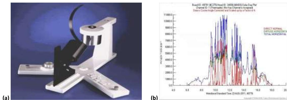
**Figure 6:** a) A view of the MFRSR showing the sensor head and the rotating shadowband driven by motor, mounted in a same base, b) Measurements of the three solar radiation components at the broadband channel of the MFRSR during 22th August 2011.
