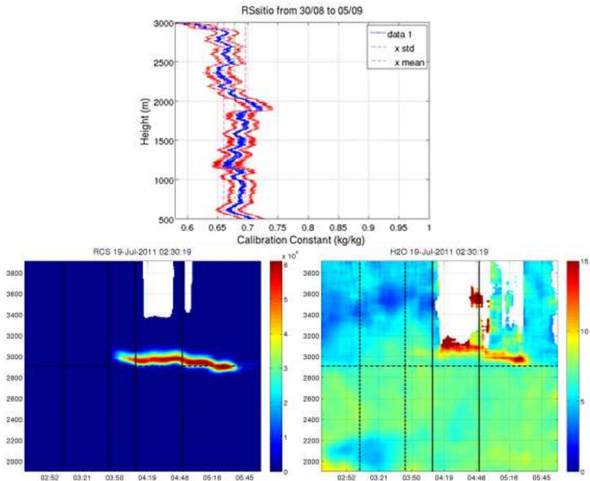
**Figure 4:** LEFT: Ratio between uncalibrated Lidar profiles and reference water vapor measurements for collocated soundings. Data shown is the average of 8 sounding between August 30<sup>th</sup> and September 5<sup>th</sup> 2011. CENTER: range corrected signal and (RIGHT) water vapor mixing ratio (right, g/kg) around a cloud.
