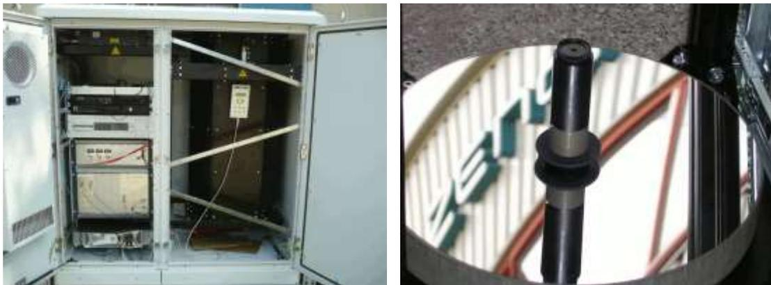
**Figure 2:** A view of the LIDAR cabinet showing the telescope, laser and acquisition system is shown. On the right, a photo of the inside of the telescope shows the primary mirror and the field stop.
